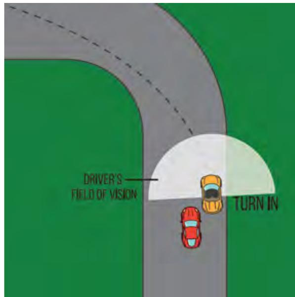
The diagram above shows at the lead car's turn in point the overtaking car has yet to get even with the A pillar and into the peripheral vision of the lead car. The overtaking car is in a blind spot. Do not pass, unless the lead car is much slower and gives racing room.
