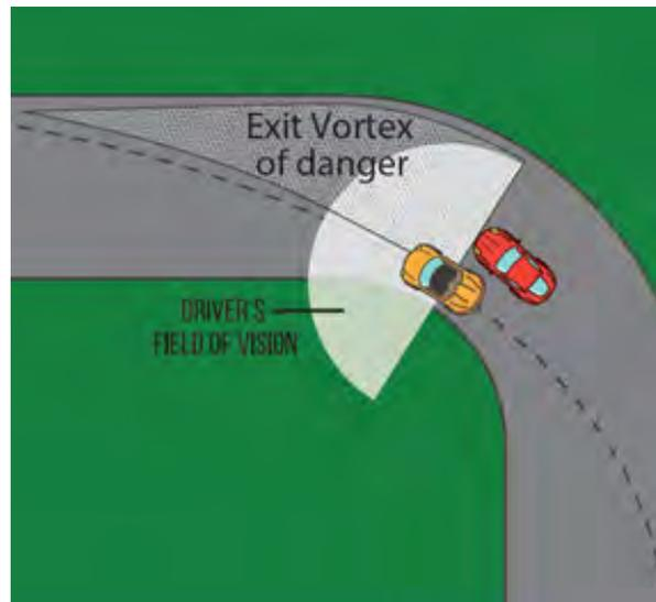
The Exit Vortex of Danger is a triangle inscribed by the apex, the track-out point of the lead car, and the outside edge of the road. When attempting a pass on the outside, be aware of the Exit Vortex of Danger, and back out of it if not in the lead car's vision. It's too late to safely pass. The hole you see on the outside is closing rapidly, you are in a blind spot, there will likely be contact, and it will be your fault.
