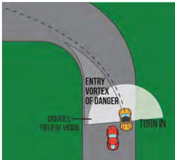
The Entry Vortex of Danger is a triangle inscribed by the turn-in point of the lead car, the apex, and the inside edge of the road. When overtaking, keep out of the Vortex of Danger. It's too late to pass. The hole you see is closing rapidly, you are in a blind spot, there will likely be contact, and it will be your fault.
