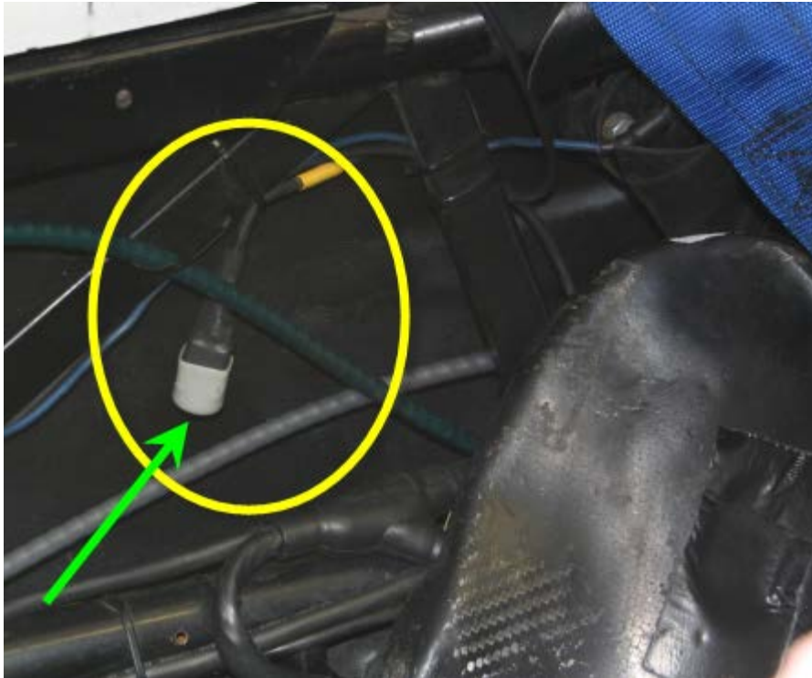
Driver's right - this one has a cover on it to keep the crud out
