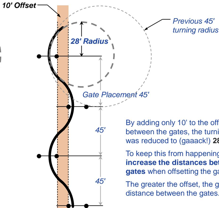
By adding only 10' to the offset between the gates, the turning radius was reduced to (gaaack!) **28 feet!**
