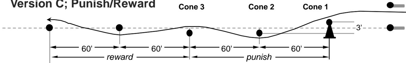
Note: Cones 1 & 2 are offset 3' the hard way with cone 3 offset 1.5' the easy way. This opens up a "Lotus freeway" through the last 3 cones of the slalom. To make the punishment bearable, be sure to allow adequate set up area prior to the punishment, otherwise the punishment becomes painful
