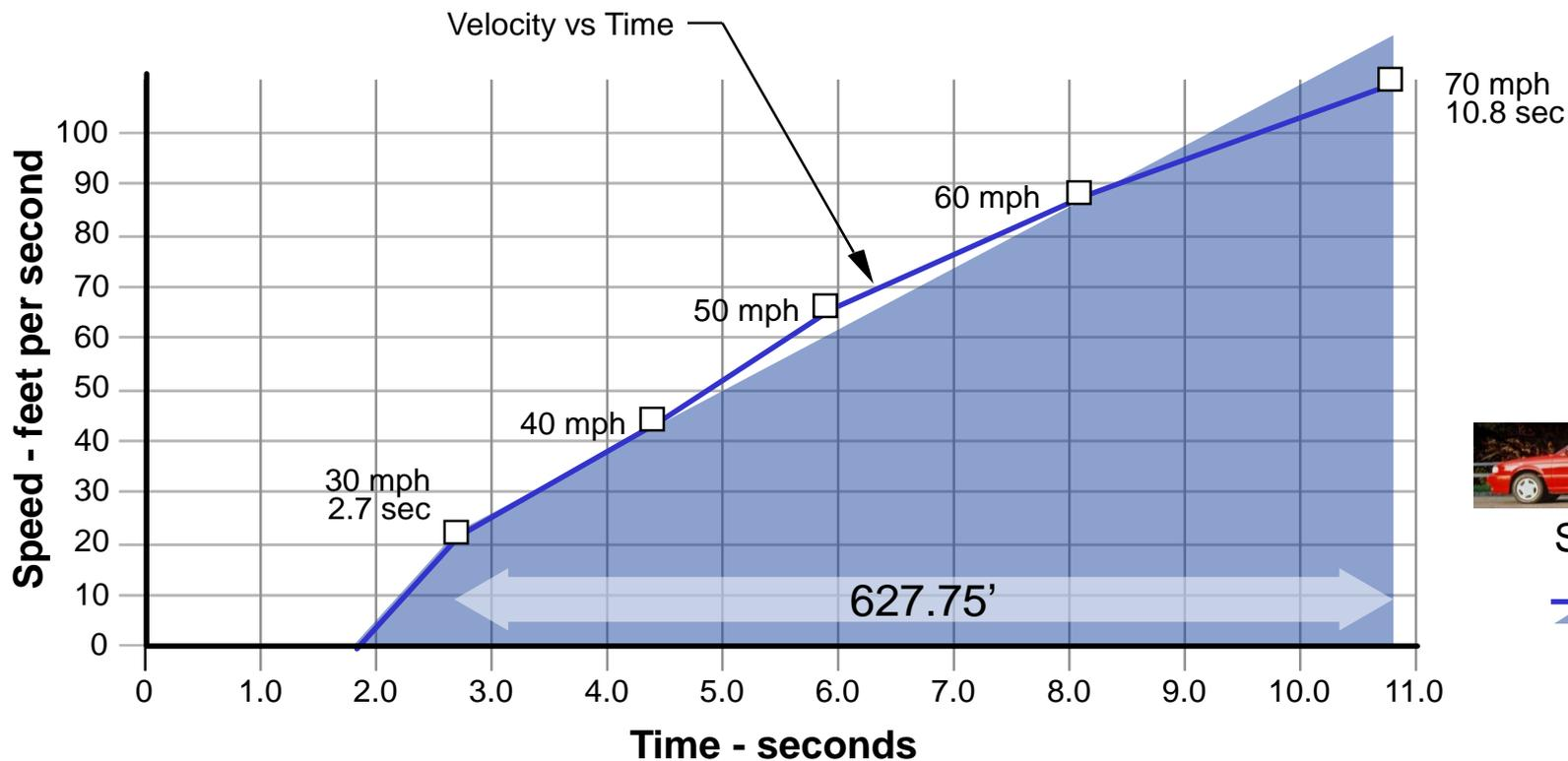
*Under full acceleration from 30 to 70mph, the Sentra will travel 627.75 feet in 8.1 seconds*
