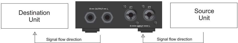
Fig. 1. Signal Flow through the PVC
