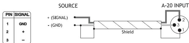
Fig. 3b Unbalanced Wiring Diagram
