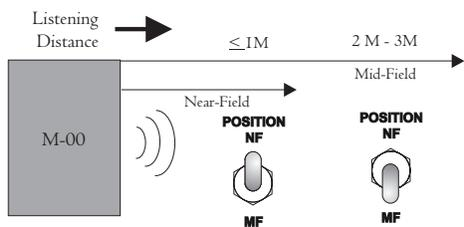
Fig. 4 Position Control Settings Diagram
