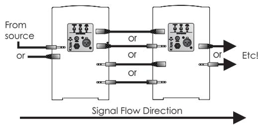
Fig. 7 Daisy Chain Connection Diagram
