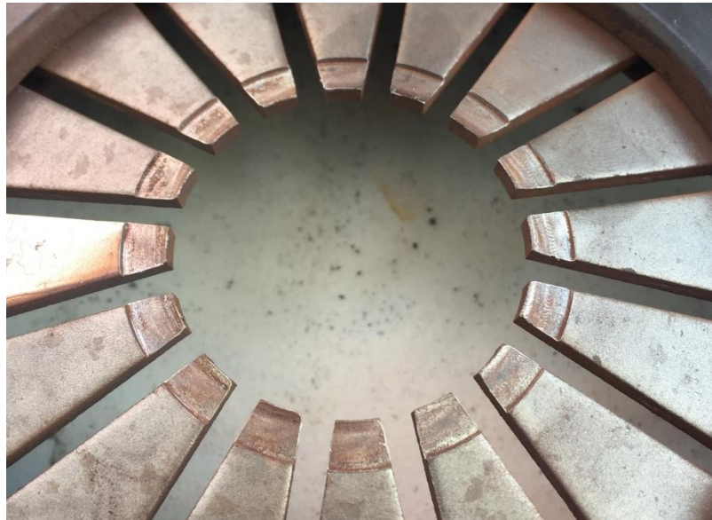
Figure 3: Heavy wear on clutch fingers
