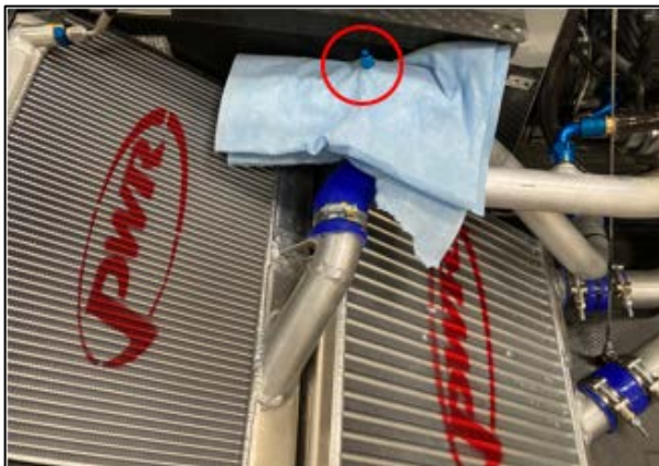
Left hand side radiator outlet bleed
